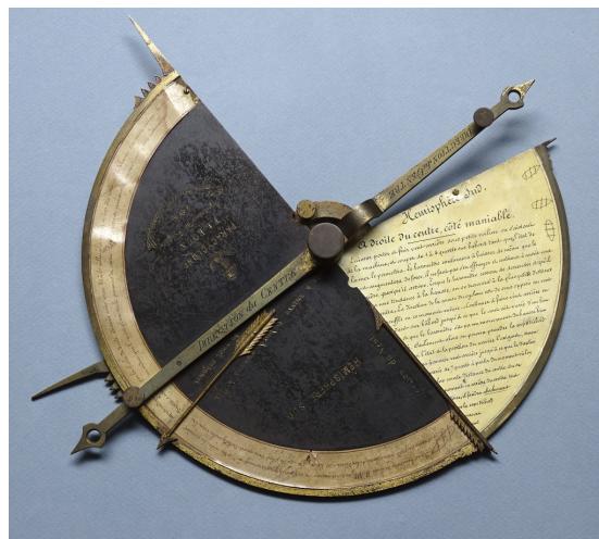
Combined cyclonometer and typhoon-barometer produced by Schmidt & Ziegler in Remscheid around 1915. Designed by Jose Maria Algue, director of the Manila Observatory.
